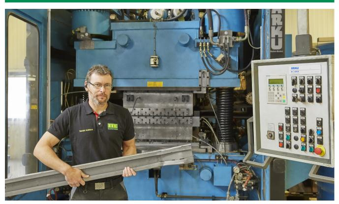
ITE can build and run tools for materials between 0,1mm to 12mm thickness from coil and sheets, in various metallic materials. ITE can offer Robot- and manual Nutwelding and/or assembly operations.
